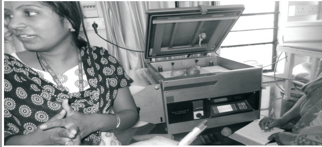
Figure 3. Vacuum Packaging Machine for Enhancing Storage Time and Quality of Food Products
